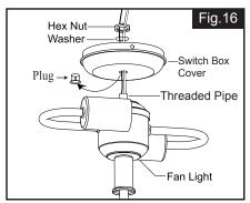
Remove the plug from the switch box. Remove the nut and lock washer from fan light. Attach the fan light to the switch box by threading the fan light wires (black and white) and remove threaded pipe through the hole of switch box and then secure them onto the switch box with hex nut & washer. Be sure it is tight enough to prevent light kit from vibrating loose.
