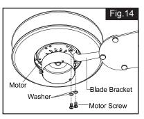
Remove the motor screws and washers from the fan motor assembly. Secure blade brackets to the motor with washers and motor screws.
