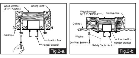
Tighten the hanger bracket to the outlet box with two mounting screws.(**Make sure the outlet box is securely installed so that it will be able to support at least the fan weight.**) Attach the safety cable hook to the ceiling with the dry wall screw and washer, and make sure the safety cable hook is covered by the fan canopy. **WARNING: MOUNT ONLY TO AN OUTLET BOX MARKED "ACCEPTABLE FOR FAN SUPPORT"!**
