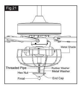
Install the metal shade, rubber washer and metal washer upward through the threaded pipe and secure with hex nut. Then attach the end cap to the metal shade and secure it with finial. Take care to align the holes on the metal shade and the end cap, so that the pull chains pass through and move freely.
