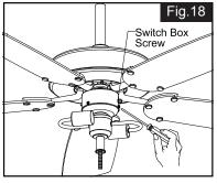
Secure the switch box cover onto switch box with the switch box screws.
