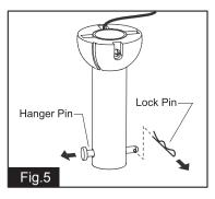
(For downrod mount only): Remove the lock pin and take off the hanger pin.
