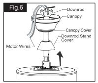
(For downrod mount only): Thread the motor wires through the downrod stand cover, decorative cap (Making sure the smooth side of decorative cap is facing downward), canopy and downrod.
