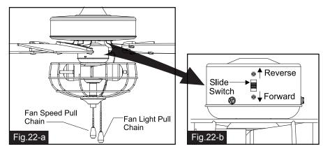
The slide switch on switch box sets direction of fan rotation. Select the desired direction of fan rotation.Push the slide switch left for "Forward" and right for "Reverse".
