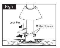
(For downrod mount only): Tighten the two collar screws. Slide lock pin into hanger pin until it is locked into position.
