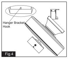
(For ceiling mount only): Raise the fan and place the canopy on the hanger bracket hook for wiring.
