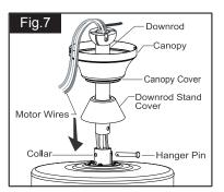
(For downrod mount only): Loosen the collar screws out part way. Insert the downrod into the collar. Slide hanger pin through holes of collar and downrod.
